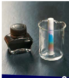
Figure 6.1 A simple chromatogram. One end of this chalk was dipped in black ink before being placed in the beaker of water. The black ink separates into its different coloured components as it rises up the chalk.
