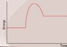
Figure 15.24 Energy level diagram for the production of hydrogen iodide.
